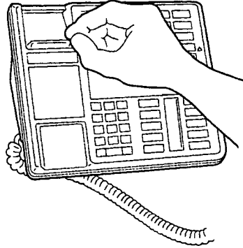
Installing the receiver clip
